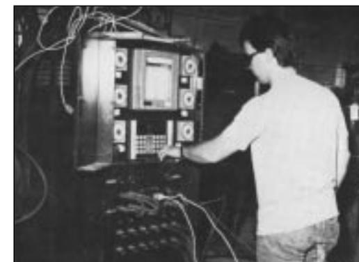
FIGURE 2: Technician programming a controller to post weld heat treat a small valve in the Vogt Metallurgy and Welding Department Laboratory
