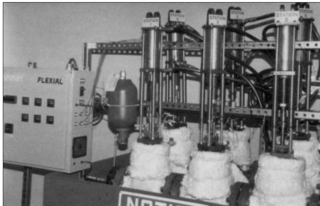
Six Flexial Reactive Seals™ under life test in Vogt 3-inch, API-602 forged steel gate valves at 1250 psi and 425°F. Test sponsored by Advanced Research Projects Agency.
